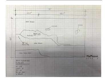
A drawing was made of the excavation's south wall. Known as a profile, it documents different layers of soil visible.
